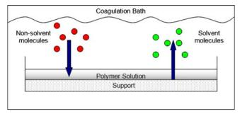
**Fig. 1.** Schematic illustration of the mass transfer of solvent and nonsolvent occurring during immersion precipitation (adapted from: Pereira *et al.* (17))
