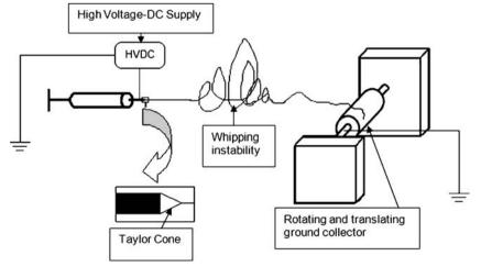
Fig. 2. An overview of the electrospinning process (adapted from: Sill and von Recum (22))
