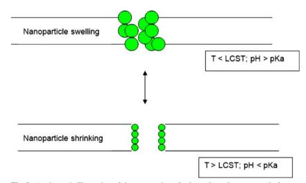
**Fig. 8.** A schematic illustration of the permeation of solutes through a nanoparticulate thermo- and pH-responsive membrane (adapted from: Zhang and Wu (114))
