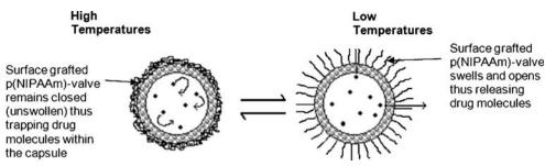
**Fig. 4.** Schematic illustration of a capsule membrane that has been grafted with polymers functioning as a permeation valve (adapted from: Okahata *et al.* (67))
