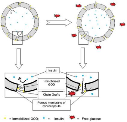
**Fig. 6.** Schematic representation of glucose-responsive microcapsules prepared with a porous membrane containing functional gates. Pores consist of GOD and pH-responsive PAA chains that, upon exposure to glucose, allows for the opening of the pores thus releasing insulin (adapted from: Chu *et al.* (76))
