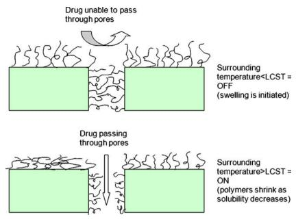
Fig. 5. 'On-off' valve mechanism of polymeric brushes grafted onto porous support (adapted from: Lue *et al.* (6))
