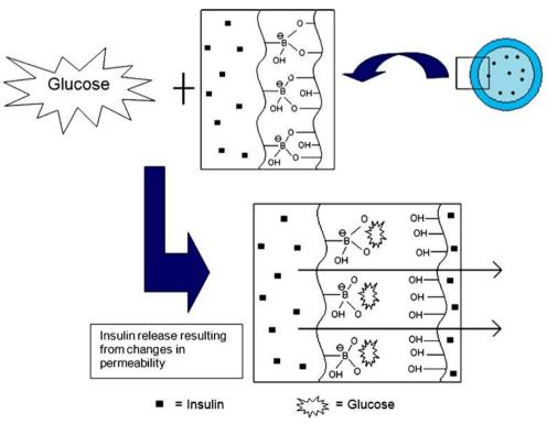
Fig. 7. A glucose-responsive insulin-releasing system based on PVA/poly(NVP-co-BPA) (adapted from: Kitano et al. (51))
